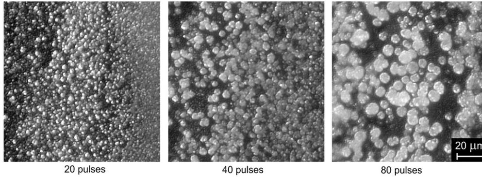
Fig. 6. Microscope pictures of deposition grains after 20, 40 and 80 laser pulses. Fluence = 2 J/cm<sup>2</sup>. Blobs are result of coagulation of 2 μm size balls.
