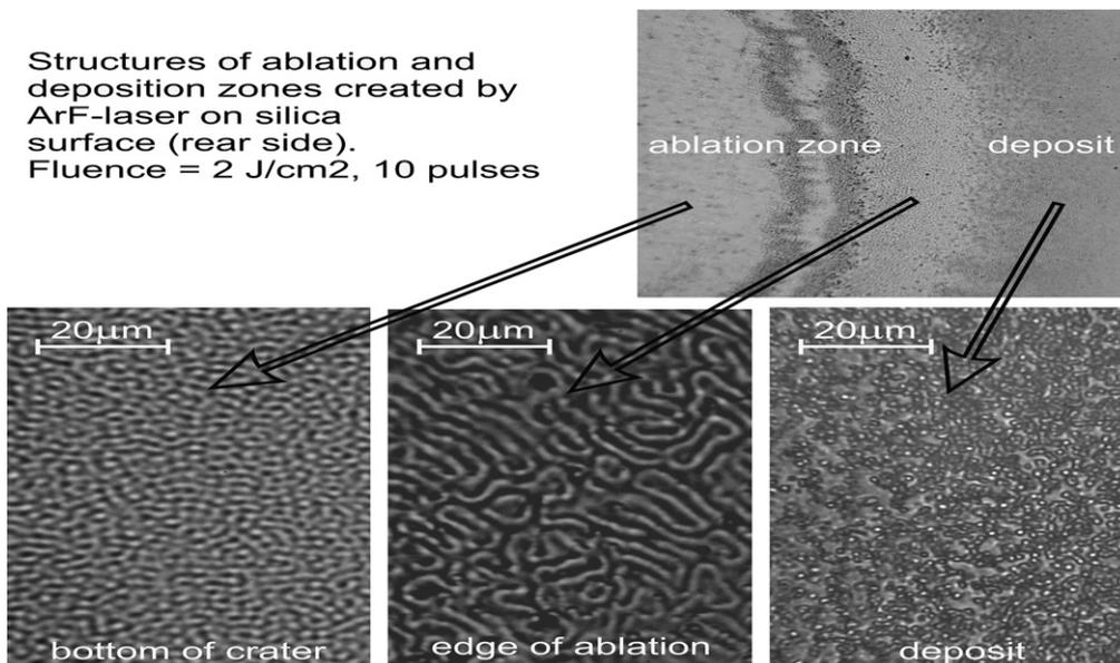
Fig. 5. Structures of ablation and deposition zones.
