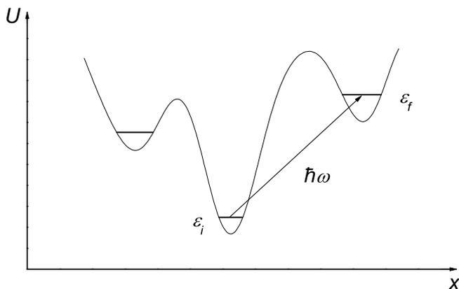
Fig. 2. Light induced electron transition between different potential wells (traps).
