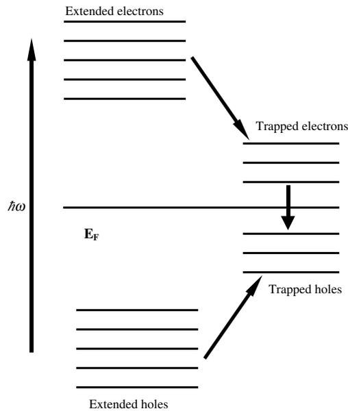
Fig. 1. Extended and trapped electron and hole states in random media.
