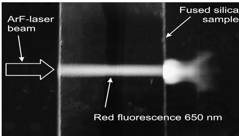
Fig. 4. Fluorescence trace and ablation plume in a fused silica samples under ArF-laser irradiation.
