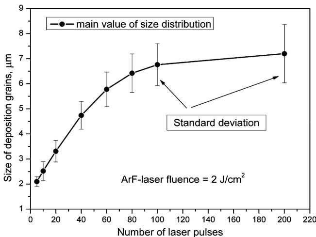
Fig. 7. Grain size vs. number of laser pulses.
